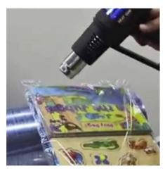
Two sides of the package are sealed simultaneously saving time and energy. A heat shrink gun (not included) shrinks the film to create a sparkling, tightly wrapped package. The VHLIB uses centrefolded PP, PVC and PE shrink film up to 0.05mm thick. The seal timer is adjustable from 1 to 3 seconds. Each sealer includes a film roll dispenser.
